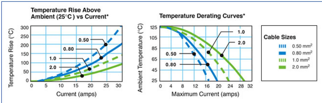
\* The test data is based on single circuits in free space and was generated using a "lumped resistance" model. The data presented here does not account for all variables that would be present in an actual application. Delphi Engineering can model customers' specific applications upon request. For additional detailed product performance, visit our website at [delphi.com/connect](http://delphi.com/connect) or call [1] 248.813.2330.
